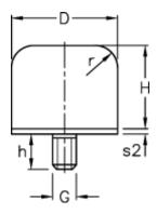
D = 125 s2 = 4 G = M16 H = 100 h = 36 Load capacity F (kN) = 150.0 Load capacity f (mm) = 55 Load capacity W (J) = 2240 r = 25.0
